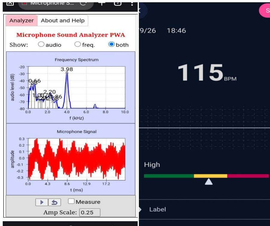
Figure 5: Frequency spectrum analysis of input sound correlated with real-time PPG heart rate measurement.
