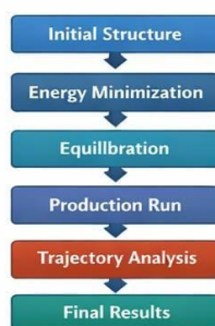
Fig. 2: Workflow of Molecular Dynamics Simulation
