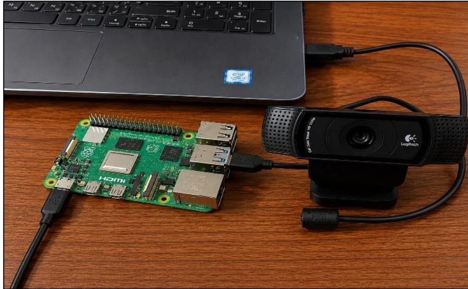
Fig. 2: Hardware Setup — Raspberry Pi 4 with USB webcam configured for real-time attendance
