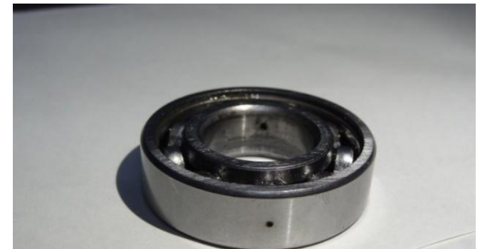
Figure 4.8 Inner-outer defects (0.7 mm holes)
