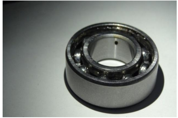
Figure 4.6 Inner race defect (0.7 mm hole)
