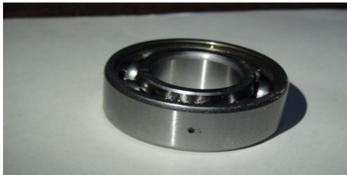
Figure 4.5 Outer race defect (0.7mm hole)
