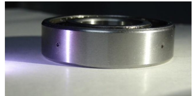
Figure 4.9 Two-outer race defects at 90 degree (0.7 mm holes)
