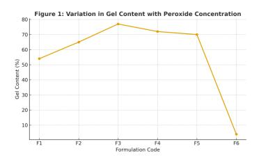
These results align with observations by Patil *et al.* (2021, J Indian Chem Soc), who reported a 30 % rise in gel content for peroxide–TAIC systems in LDPE. The synergy between silane grafting and radical crosslinking accelerated network connectivity, a mechanism also supported by the model predictions.
