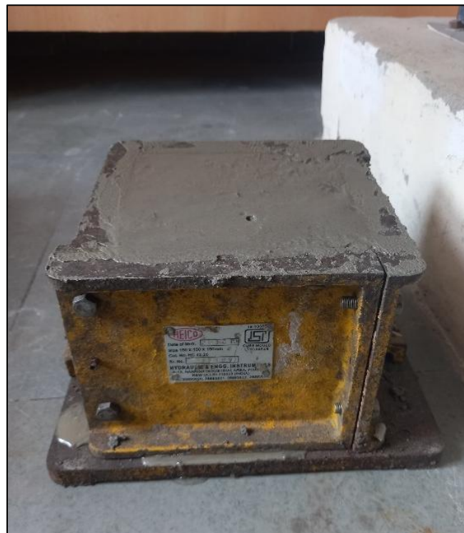
Figure 5: Concrete mix poured into the mold
