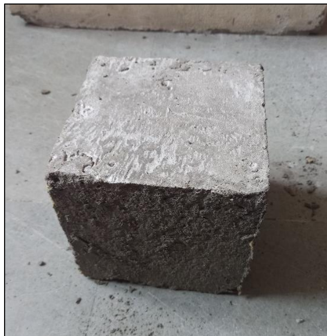
Figure 7: Concrete cube after curing
