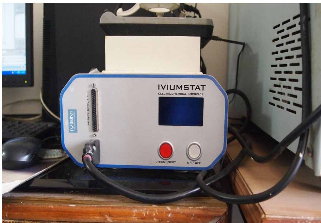
Plate 7: IVIUM Potentiostat Galvanostat using a triple electrode assembly
